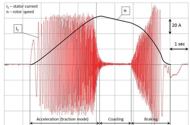
**Figure 13:** Change of phase current and frequency of rotor rotation of DMG with alternation of modes of WP prototype: acceleration-coasting-braking
