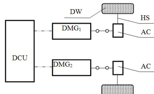
**Figure 1:** Design layout of WP with two half shafts, angle-change gearboxes and mechanically independent drives DCU – control unit of the drive; DMG – drive motor-generator; ACG – angle-change gearbox; MCD – mechanical coupling device of DMG and ACG; HS – half shaft; DW – drive wheels.
