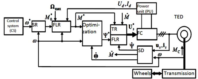
**Figure 2:** Generalized functional layout of TED control system on the basis of IM and CVUJ
