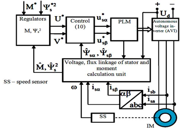
**Figure 4:** Functional layout of induction electric drive with DMC
