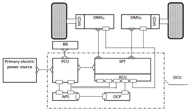
**Figure 7:** Structural layout of functional components of DCU prototype
