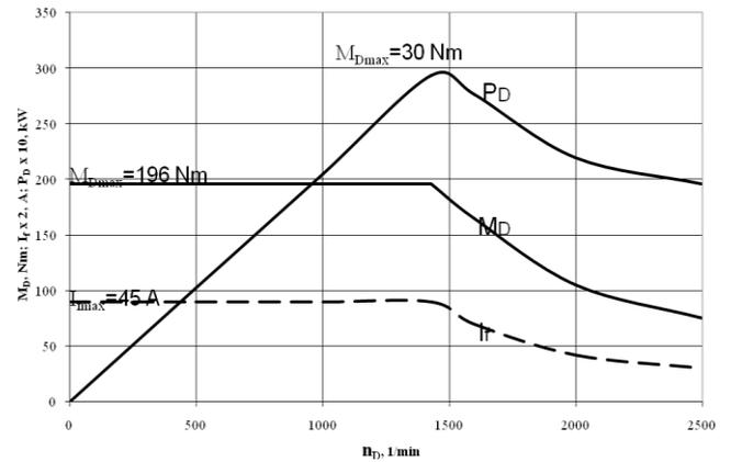
**Figure 11:** Relationship between moment, shaft power and phase current of DMG of WP driver and the frequency of rotation of the rotor
