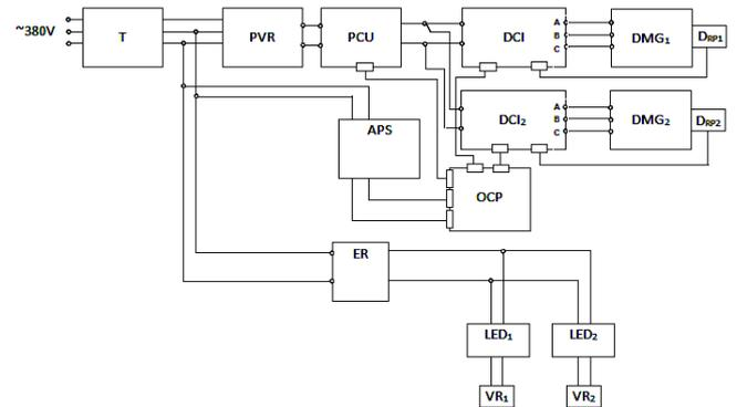
**Figure 8:** Functional electric layout of the testing bench for experimental studies of WP and DCU, where: T – controlled transformer; PVR– power voltage rectifier; PCU – power commutation unit; APS – auxiliary power source; DCI – DC inverter; OCP – operating control panel; DMG – drive motor-generator; ER – excitation regulator of LED; LED – loading electric device; VR – voltage regulator of LED; D<sub>RP</sub> – rotor position sensor.
