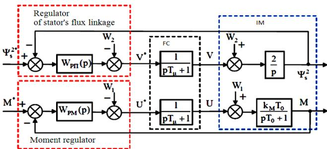
**Figure 3:** Structural layout of closed circuits of regulation of flux linkage of stator and IM moment
