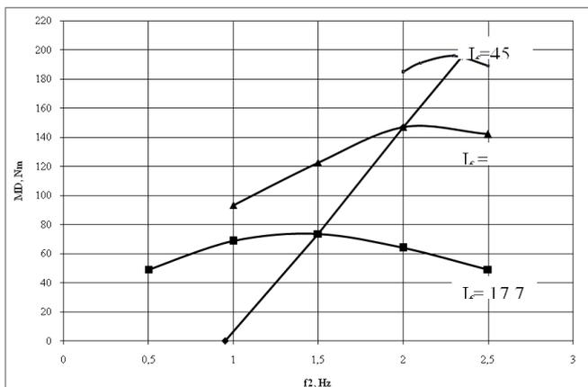
**Figure 9:** Relationship between torque of DMG and  $f_2$  frequency with constant values of  $I_f$
